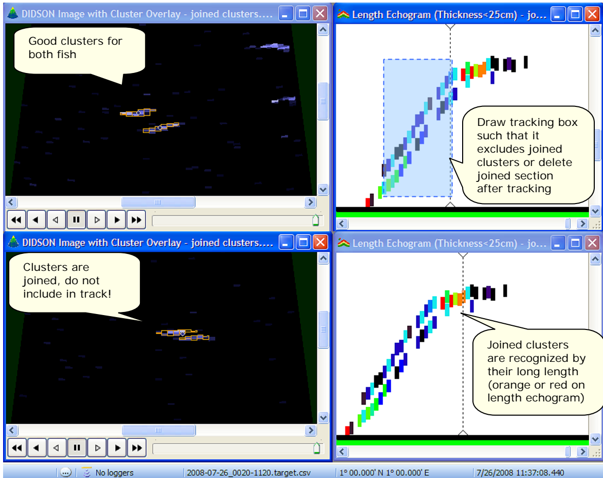
Figure 14. With closely spaced fish make sure the tracks do not include joined clusters.
