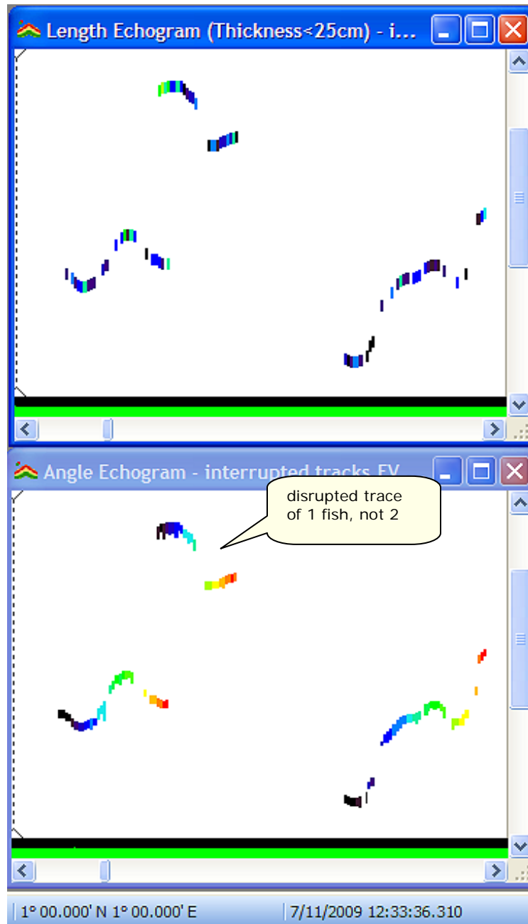
Figure 4. Not all fish traces are as clean and solid as those shown in the previous figure. Depending on the tidal stage and fish behavior the traces may be disrupted. This happens especially when the fish change range rapidly. Note on the Length Echogram it is impossible to tell whether the two traces at the top belong to one fish or two. Looking at the progression of the colors on the Angle Echogram it is obvious that it is the disrupted trace of one fish. In total, this echogram snippet shows the disrupted traces of 3 fish. To determine whether a group of echoes belongs to one or multiple fish one can also review the DIDSON video. However, usually it is immediately obvious on the Angle Echogram, which can save a considerable amount of time.
